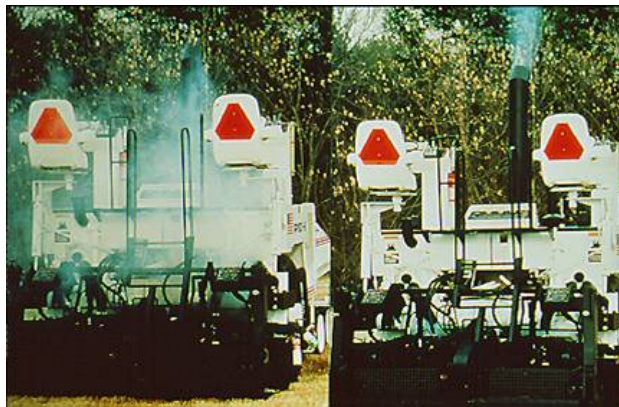
Figure 1. Photograph of an asphalt paver before (left) and after (right) an engineering control was installed to reduce asphalt fume exposures.
